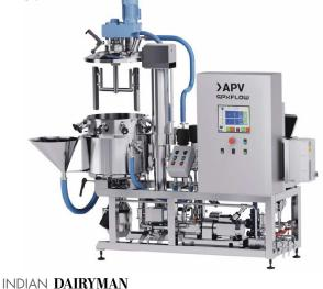
Vacuum-mixing: For low viscosity products like infant formula and plant-based products. It uses external recirculation and scales up to our Flex-Mix<sup>™</sup> Instant mixer.
