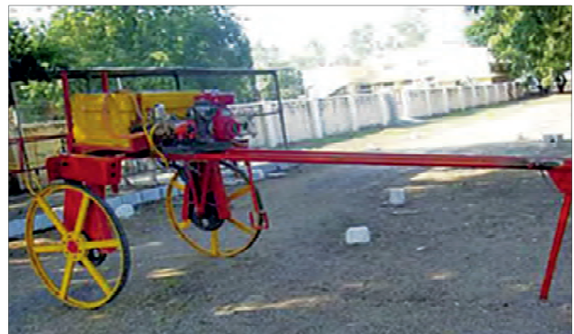
Fig. 2: Spraying of pesticides with modified bullock cart (Source: AICRP, University for Agricultural Sciences, Karnataka).
