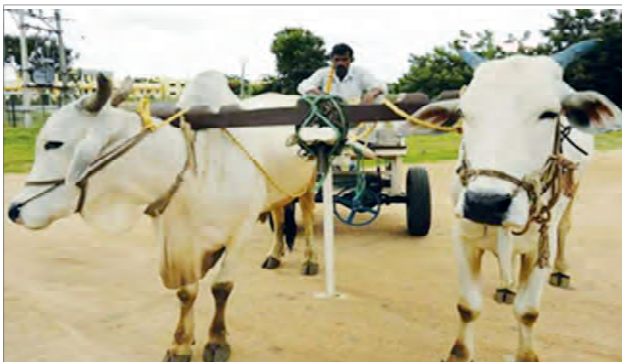
Fig. 1: University of Agricultural Sciences, Raichur, Karnataka, has developed a bullock cart-mounted device that generates electricity from the movement of the cart (Photographs courtesy: All India Coordinated Research Project on Increased Utilization of Animal Energy) (Source: https://www.downtoearth.org.in/agriculture/bullock-turn-the-return-of-the-bullock-to-india-s-farms-81805 ).
