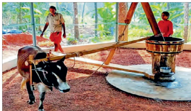
Fig. 7: Traditional method of extracting oil using the mechanical power of bullocks
