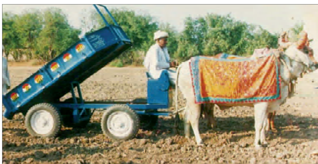
Fig. 5: Amrutbhai Agrawat, Gujarat farmer, with his tilting bullock cart (Source: http://www.nif.org.in/public/upload/innovation/6th/490-multiple-agricultural-machineries.pdf )
