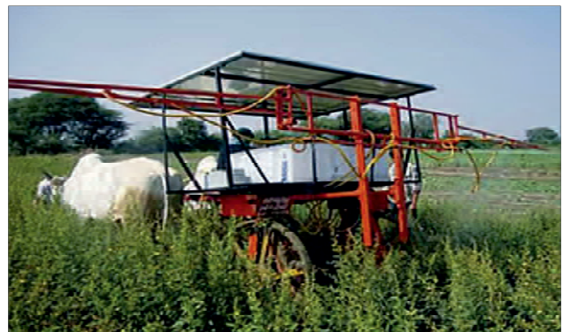
Fig. 3: Spraying of pesticides with bullocks using energy generated by solar panels mounted on bullock cart (Source: AICRP, University for Agricultural Sciences, Karnataka).
